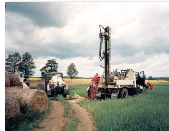
Drilling shot holes during Polonaise experiment, May 1997.
