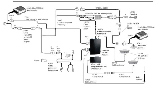
**Note** – For installation of the TrueTracker joystick with manual steering, see the document 92405-06-E05.
