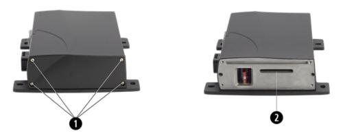
Insert the AG-815 blade connector (2) into the radio expansion slot of the TM-200 Module.
