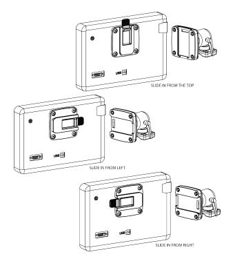
The quick release tab should point in the opposite direction from the direction you will slide the display out of the mount.
