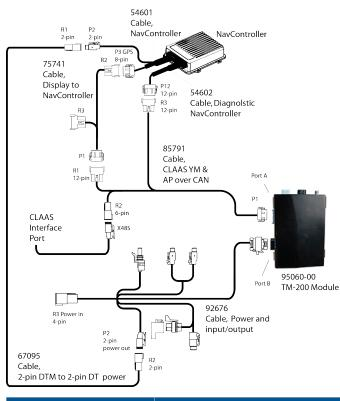
Use this diagram to connect the CLAAS Jaguar forage harvester.
