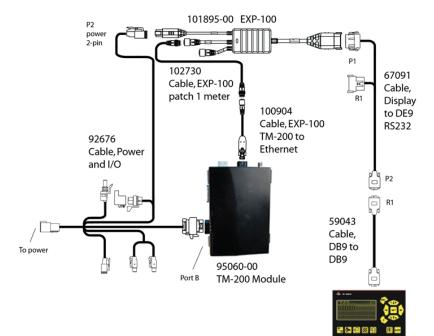
This diagram shows the connections for the Hardi 5500 controller with serial variable rate and radar output.
